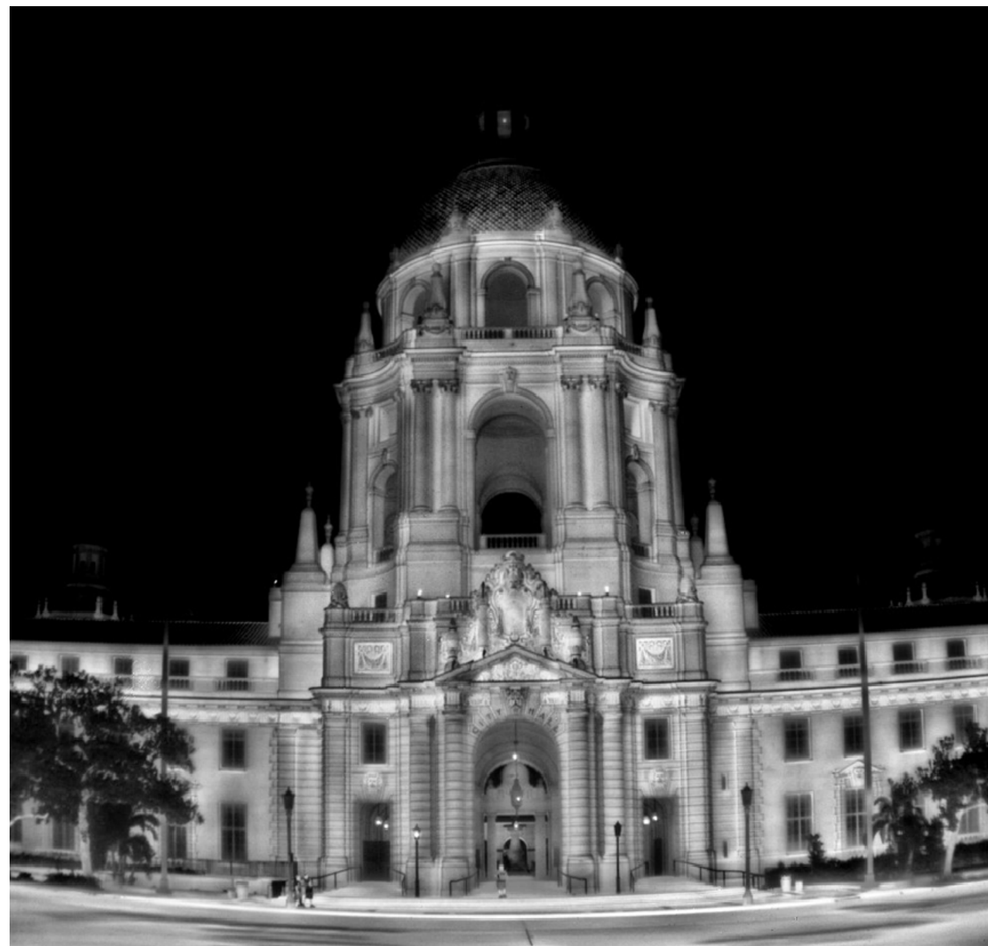
Fig. 4. IR image of Pasadena City Hall taken with a JPL BIRD FPA.
